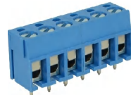
DAHM500 Pitch 5.0mm Poles 2p,3p PCB screw terminal blocks, horizontal wire inlet
